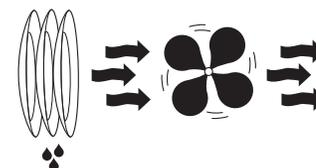
If the **HEATED DRY** option is selected, the drying fan will run during the drying portion of the cycle and up to 2 hours after the **CLEAN** light is on, depending on the selected wash cycle. If the **HEATED DRY** option is not used, the **CLEAN** light will come on at the end of the final rinse and the fan will run up to 4 hours, depending on the selected wash cycle.
