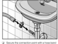
Secure the connection point with a hose band clip. Drainage into a wash basin
