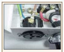
**<u>HINT</u>**: Bosch dryers include a NEMA 6-15R outlet which the washer **NEMA 6-15P** 240V, 15A, 3-wire plug can be plugged into.
