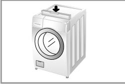
1. Adjusting the washing machine level properly prevents excessive noise and vibration.
