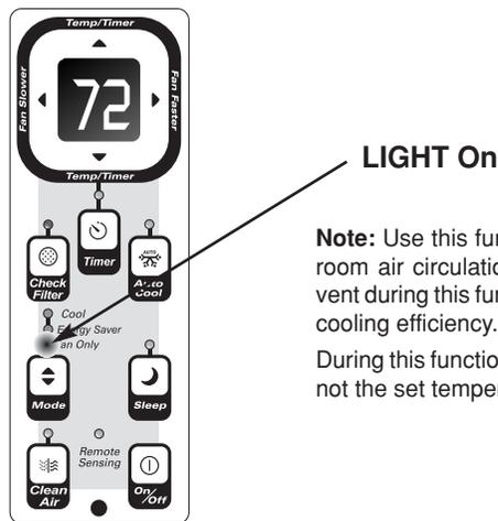
**Note:** Use this function only when cooling is not desired, such as for room air circulation or to exhaust stale air. (Remember to open the vent during this function, but keep it closed during cooling for maximum cooling efficiency.) You can choose any fan speed you prefer. During this function, the display will show the actual room temperature, not the set temperature as in the cooling mode.
