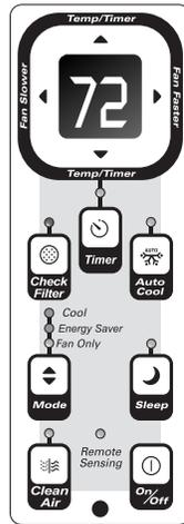
**Note:** Tap or hold either up (  $\wedge$  ) or down (  $\vee$  ) button until the desired temperature is seen on the display. This temperature will be automatically maintained anywhere between 60°F (16°C) and 90°F (32°C). If you want the display to read the actual room temperature. See “To Operate on Fan Only” section on Page 7.
