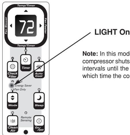
**Note:** In this mode, the fan will continue to run for 3 minutes after the compressor shuts off. The fan then cycles on for 2 minutes at 10 minute intervals until the room temperature is above the set temperature, at which time the compressor turns back on and cooling stars.
