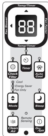
A 2 Digit Display is used to indicate the Fan Speed setting, from 10 through 99. When the “SLOWER” button is pressed the motor speed will slow down at multiple intervals (90 distinct settings), to a minimum setting of 10. To speed the motor up, press the “FASTER” button. The speed will increase at multiple intervals to a maximum setting of 99. After 5 seconds the control will automatically change back to displaying the set temperature.
