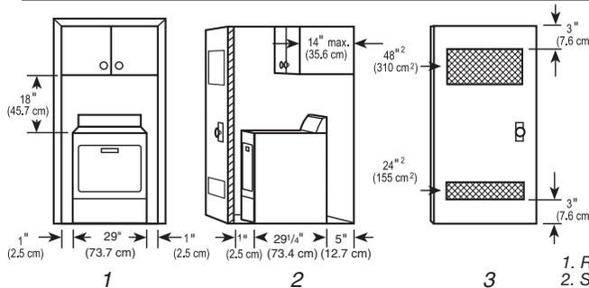
For closet installation with a door, minimum ventilation openings in the top and bottom of the door are required. Louvered doors with equivalent air openings are acceptable.
