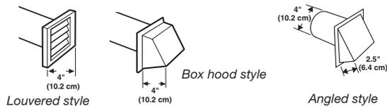
1. Select the route that will provide the straightest and most direct path outdoors. Plan the installation to use the fewest number of elbows and turns. When using elbows or making turns, allow as much room as possible. Bend vent gradually to avoid kinking. Avoid 90° turns.
