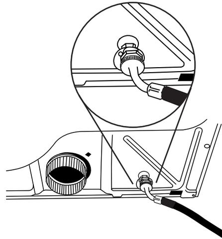
**NOTE:** Do not overtighten. Damage to the coupling can result.
