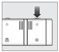
Press the button in the direction of the arrow until the flap springs open.
