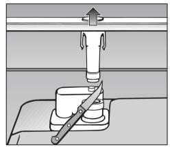
Cut off the vent cap located at the right rear of the triple filter system, as illustrated. When contacting the Technical Service, please quote the model and serial number of your appliance.
