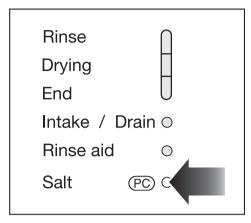
When the "Salt" indicator comes on, refill the salt after the program is finished.
