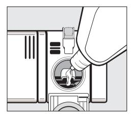
Pour liquid rinse aid into the reservoir until it its visible on the surface of the screen.
