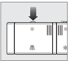
To open, press the latch on the detergent dispenser. The flap will spring open.
