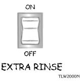
The extra rinse control is useful for detergent sensitive skin. By pressing the EXTRA RINSE to ON, the REGULAR, PERMANENT PRESS, and HANDWASH/DELICATE cycles will each provide an additional rinse. If the rinse is desired, press the switch to ON. When the extra rinse is not wanted, OFF should be selected.
