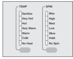
Press the "TEMP" and "SPIN" buttons until the indicator of the desired value lights.
