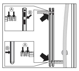
Fasten the shipping struts to the rear of the washer. Take care to insert the drill holes correctly,
