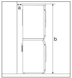
The Miele washing machine can be installed as part of a washer-dryer stack in combination with a Miele tumble dryer. An appropriate "stacking kit\*" is required.
