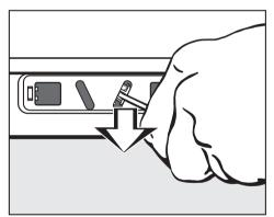
Insert a screwdriver into the notch of the right opening and pull downwards. The door will now open.
