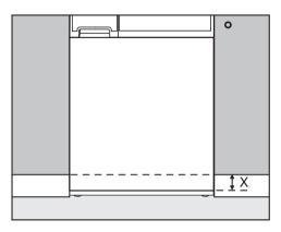
The measure **X** equals the space from the bottom of the washer door to the bottom of the adjacent cabinet.
