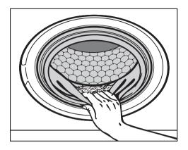
Check the folds of the door seal for any small articles which may have been trapped.
