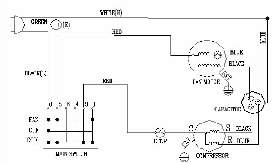
Note: The illustration is explained the wire connection of the 0.T.P of the external compressor. For the internal compressor, the 0.T.P has been connected with the compressor.
