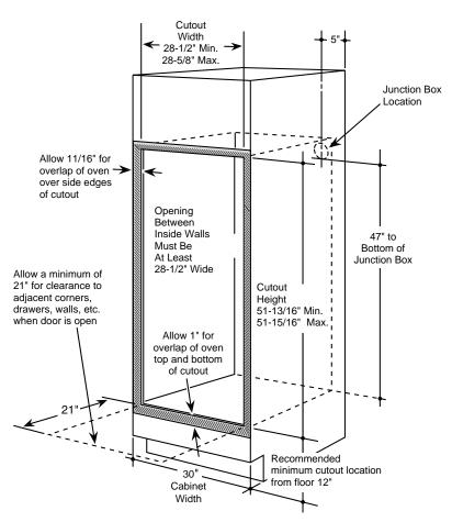
If the cabinet does not have a solid bottom, two braces or runners must be installed to support the weight of the oven. For double ovens, the runners and braces must support 275 lbs.
