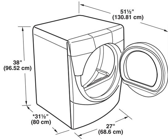
\*Most installations require a minimum 5 1/2" (14 cm) clearance behind the dryer for the exhaust vent with elbow. See "Venting Requirements."
