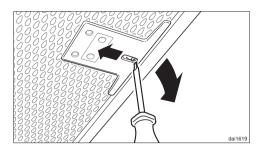
If the filter is incorrectly installed, insert a small screwdriver into the slit along its edge to disengage it from the casing.
