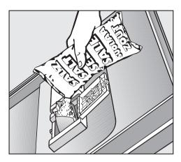
Carefully fill with salt until water runs out. The salt container holds approx.
