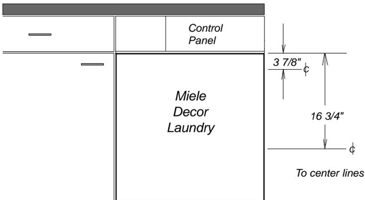
**Note:** To insure access to customer servicable features, a minimum 4" toe kick above finished floor (AFF) is required.
