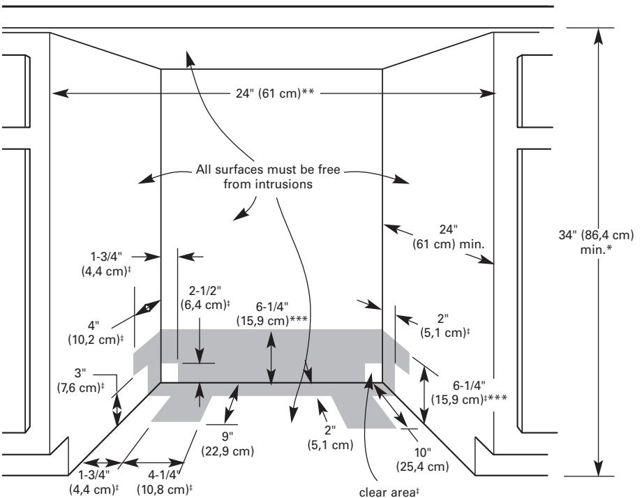
Water line entering through the left side of opening in shaded areas makes connection easier.
