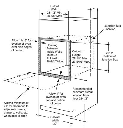
If the cabinet does not have a solid bottom, two braces or runners must be installed to support the weight of the oven. For single ovens, the runners and braces must support 150 lbs.
