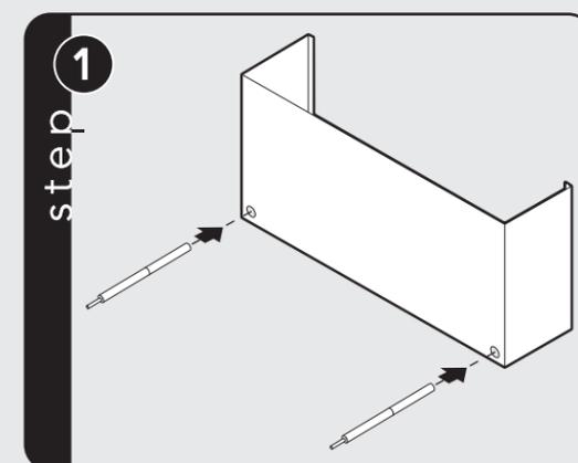
Slide rails into openings in duct cover.
