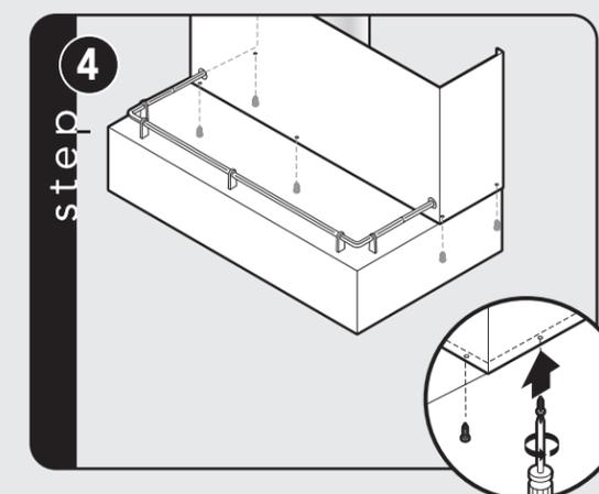
Fasten duct cover to canopy with screws provided.
