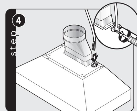
Insert 6" of electrical wiring through the top of vent hood and secure using wiring restraint. Refer to local codes.
