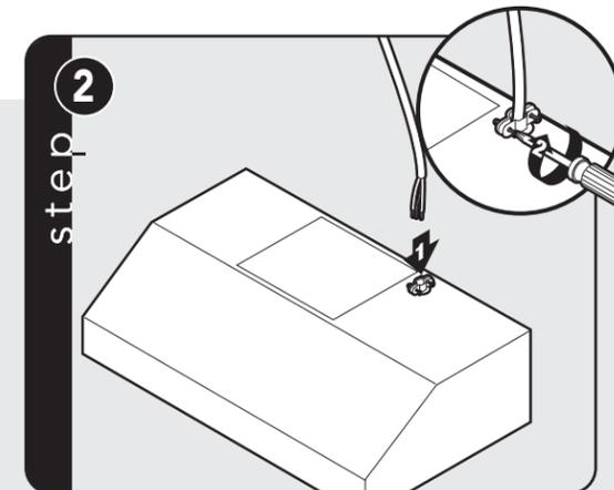
Insert 6" of electrical wiring through the top of vent hood and secure using wiring restraint. Refer to local codes.
