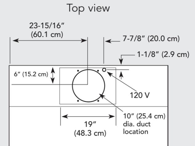
1200 or 1500 CFM Exterior Ventilator Installation for 48" models
