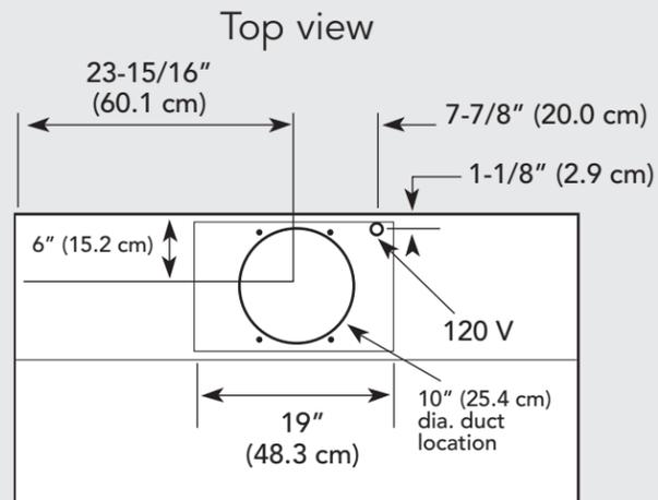
880 CFM Interior Ventilator Installation for 48" models
