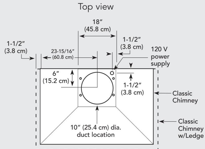
1200 CFM Interior Ventilator Installation for 48" & 51" models
