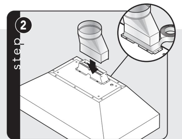
Attach transition to damper. Seal with aluminum tape.
