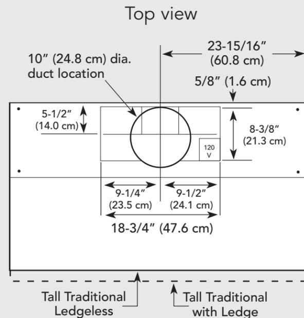
1200 CFM Interior Ventilator Installation for 48" models
