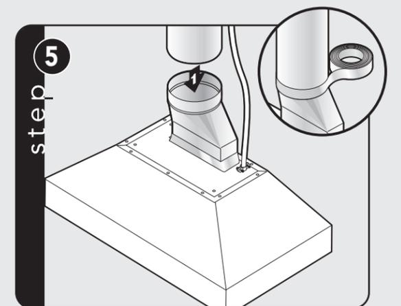
Slide duct over transition and tape around joint.
