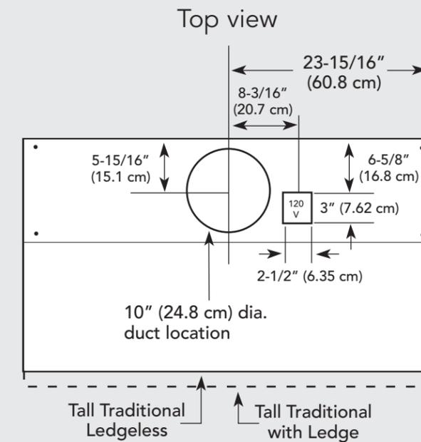
1200 or 1500 CFM Exterior Ventilator Installation for 48" models
