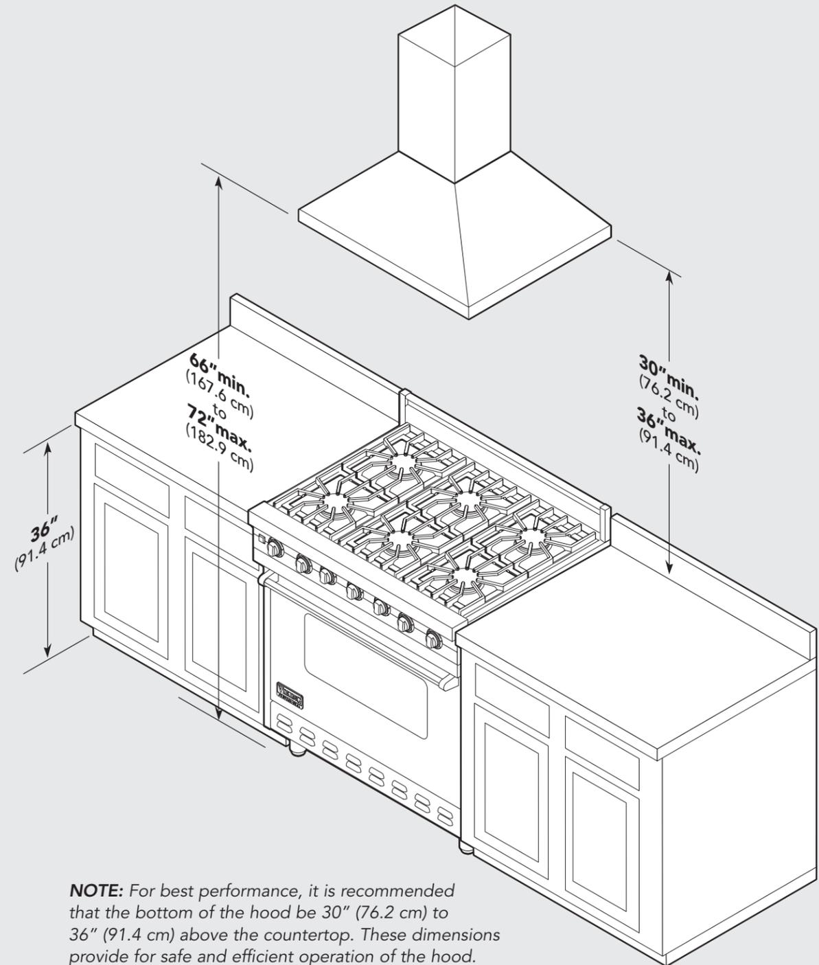
NOTE: For best performance, it is recommended that the bottom of the hood be 30" (76.2 cm) to 36" (91.4 cm) above the countertop. These dimensions provide for safe and efficient operation of the hood.
