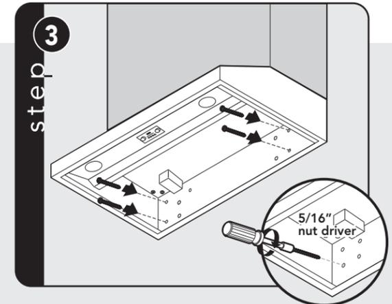
**CAUTION:** Using screws provided secure vent hood to wall. Make sure mounting screws are secured into frame. Use additional mounting screws and wall anchors, if necessary.
