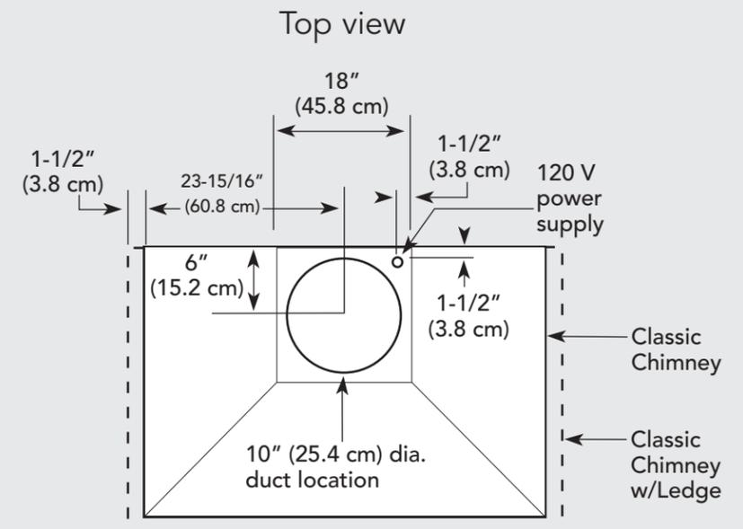
1200 or 1500 CFM Exterior Ventilator Installation for 48" & 51" models
