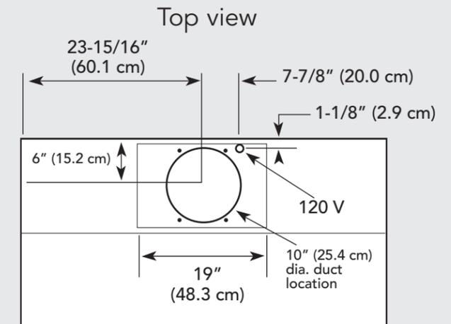
1200 or 1500 CFM Exterior Ventilator Installation for 48" models
