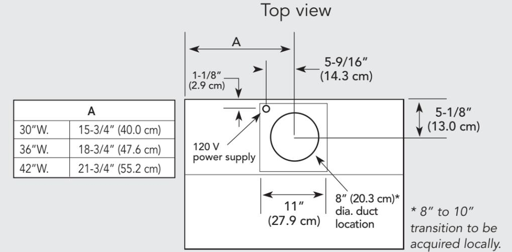
900 or 1200 CFM Exterior Ventilator Installation for 30", 36" & 42" models
