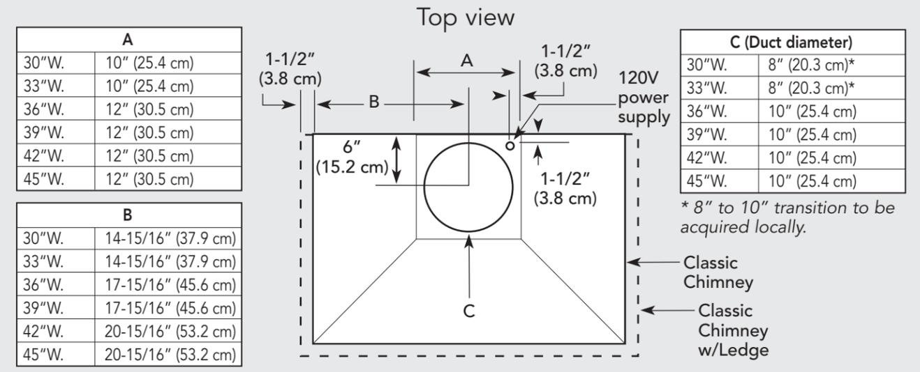
900 or 1200 CFM Exterior Ventilator Installation for 30", 33", 36", 39", 42", & 45" models
