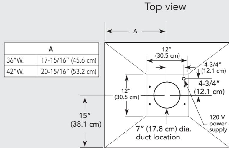
600 CFM Interior Ventilator Installation for 36" & 42" models
