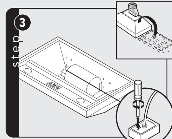
Flip hood over and remove electrical box cover.
