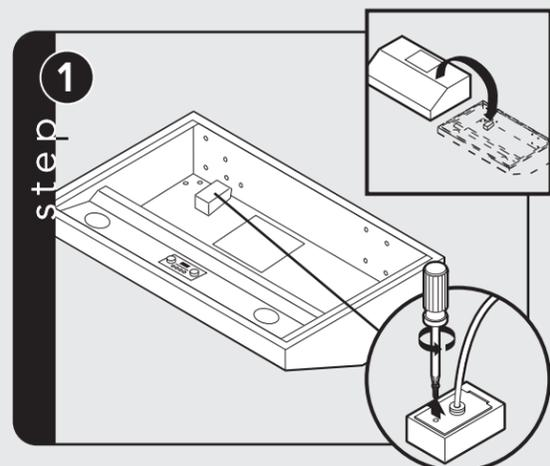
Flip hood over. Remove electrical box cover.
