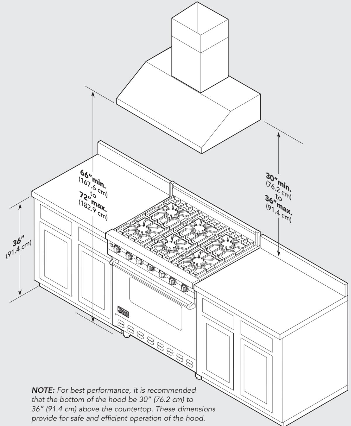
**NOTE:** For best performance, it is recommended that the bottom of the hood be 30" (76.2 cm) to 36" (91.4 cm) above the countertop. These dimensions provide for safe and efficient operation of the hood.
