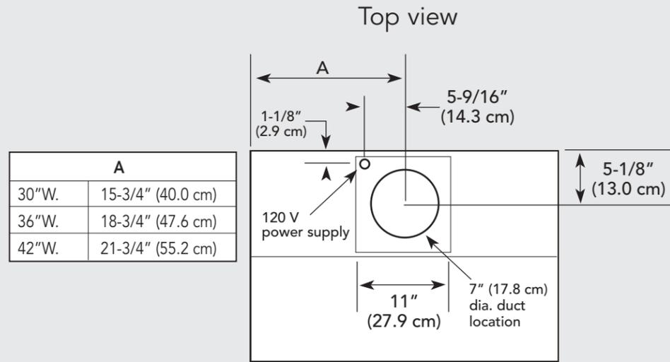
300, 440 CFM Interior Ventilator Installation for 30", 36", & 42" models
