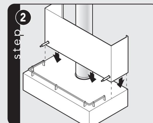
Lower duct cover into position on canopy.
