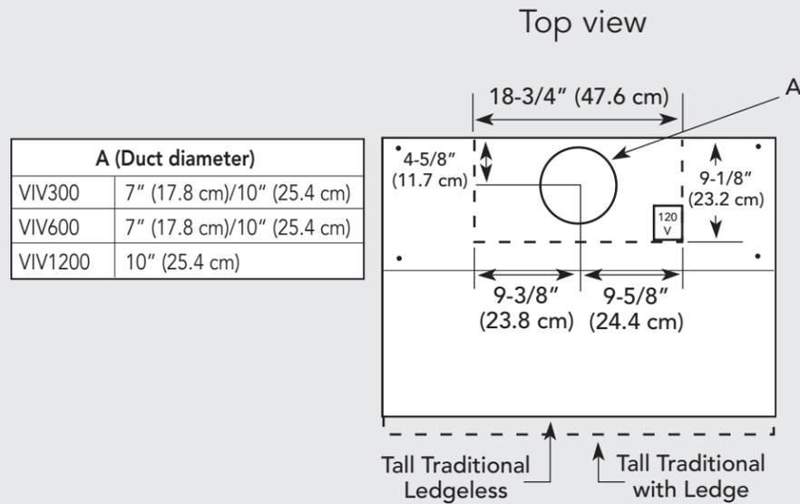
300, 600, or 1200 CFM Interior Ventilator Installation for 30", 36", & 42" models
