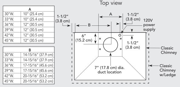
300, 440 or 600 CFM Interior Ventilator Installation for 30", 33", 36", 39", 42", & 45" models
