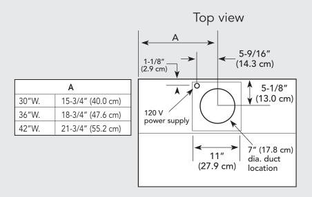
300 or 440 CFM Interior Ventilator Installation for 30", 36", & 42" models
