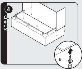
Fasten duct cover to canopy with screws provided.
