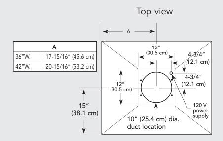
900 or 1200 CFM Exterior Ventilator Installation for 36" & 42" models
