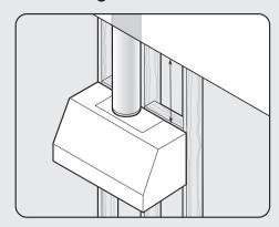
**NOTE:** Because of the weight of the hood make sure that the mounting screws are driven into the framing and not just the drywall. It may be necessary to drill additional holes in the canopy for proper alignment. Some hoods require a locally supplied wood strip for mounting. Check installation procedure of your hood on page 34 to determine if a wood strip is required.
