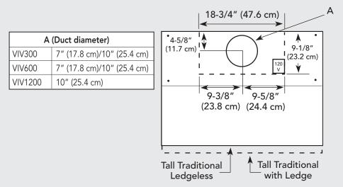
300, 600, or 1200 CFM Interior Ventilator Installation for 30", 36", & 42" models
