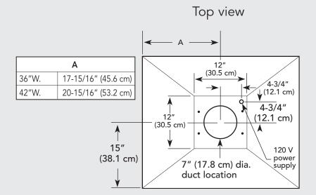
600 CFM Interior Ventilator Installation for 36" & 42" models
