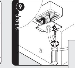
Replace electrical box cover. Make connection to breaker box.
