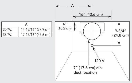
460 CFM Interior Ventilator Installation
