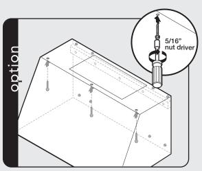
**CAUTION:** If not using a duct cover, using screws provided make sure top mounting screws are secured into soffit or cabinet frame. Use additional mounting screws, if necessary.
