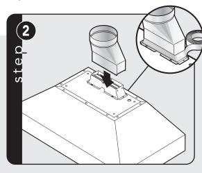
Attach transition to damper. Seal with aluminum tape.
