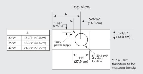
900 or 1200 CFM Exterior Ventilator Installation for 30", 36", & 42" models
