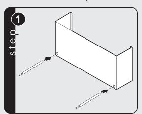
Slide rails into openings in duct cover.
