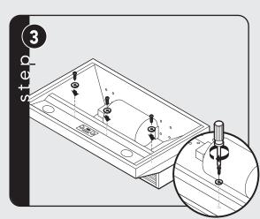
Attach with screws and lock washers provided.
