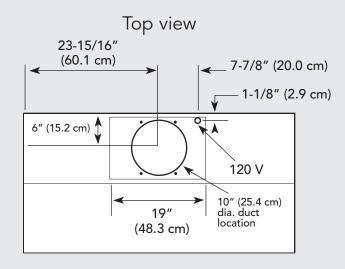
880 CFM Interior Ventilator Installation for 48" models
