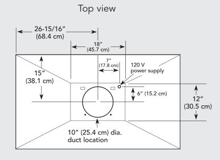
1200 CFM Interior Ventilator Installation for 54" models
