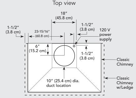
1200 or 1500 CFM Exterior Ventilator Installation for 48" & 51" models
