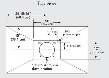
1200 or 1500 CFM Exterior Ventilator Installation for 54" models
