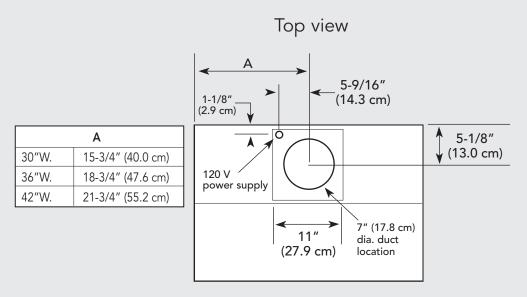
300, 440 CFM Interior Ventilator Installation for 30", 36", & 42" models
