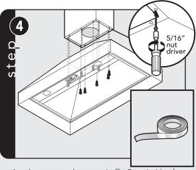
Attach canopy to duct cover/soffit. From inside of hood, seal top of hood to duct with aluminum tape.
