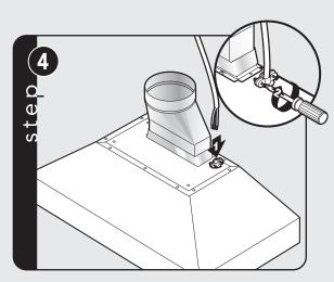
Insert 6" of electrical wiring through the top of vent hood and secure using wiring restrain. Refer to local codes.
