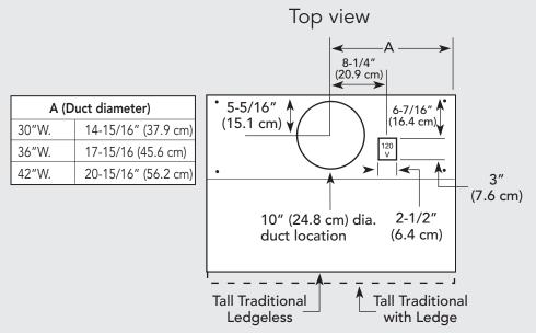
900 or 1200 CFM Exterior Ventilator Installation for 30", 36", & 42" models
