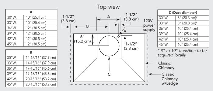
900 or 1200 CFM Exterior Ventilator Installation for 30", 33", 36", 39", 42", & 45" models
