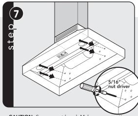
**CAUTION:** Secure vent hood. Make sure mounting screws are secured into framing using additional mounting screws and wall anchors, if necessary.
