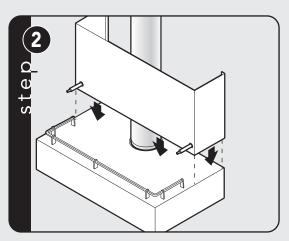
Lower duct cover into position on canopy.
