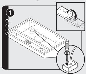
Flip hood over. Remove electrical box cover.
