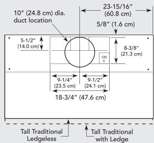
1200 CFM Interior Ventilator Installation for 48" models
