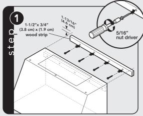
Measure down 1-13/16 (4.6 cm) from desired height of hood and secure 1-1/2" x 3/4" wood strip (not included) to wall using screws provided.
