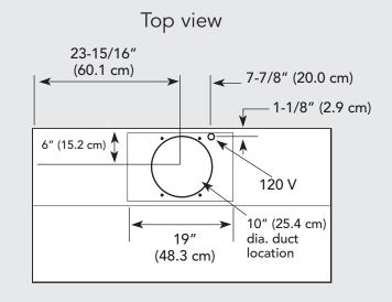
1200 or 1500 CFM Exterior Ventilator Installation for 48" models
