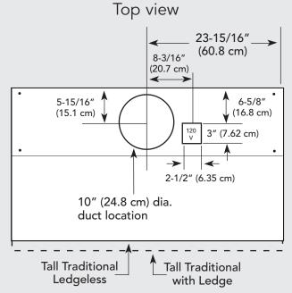
1200 or 1500 CFM Exterior Ventilator Installation for 48" models
