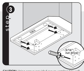
CAUTION: Using screws provided secure vent hood to wall.
