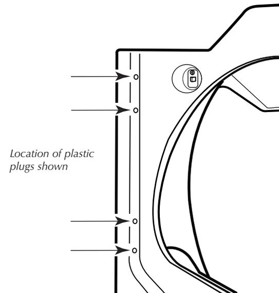
6. Install 4 plastic plugs into screw holes in the dryer left where the hinges were removed in Step 4.
