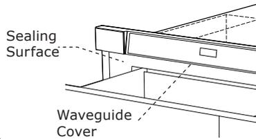
2. Remove the feature sticker, if there is one. Check the drawer for any damage, such as misaligned or bent drawer, damaged drawer seals and sealing surfaces, broken or loose drawer guides and dents inside the cavity or on the front side of the drawer. If there is any damage, do not operate the Microwave In-A-Drawer™ and contact your dealer or a DACOR AUTHORIZED SERVICER.
