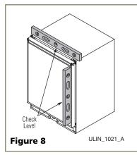
2. If the unit is not level, adjust the feet on the corners of the unit as necessary (see **Figure 9**).
