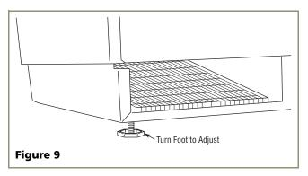
3. Check the levelness after each adjustment and repeat the previous steps until the unit is level. Go on to **Install the Unit**.
