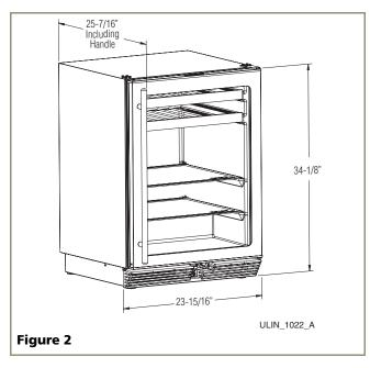
Please note that the unit has adjustable feet that can add one additional inch to height during leveling or to match adjacent cabinets (see **Figure 9**).
