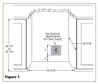
Follow the cut-out drawing in **Figure 1**. The 24-3/16" width allows 1/4" for ease in installation and removal of the unit. 24" is the cabinet depth in most installations. The unit is 23-7/16" deep including the door and *not* the handle on Stainless models (see **Figure 2**).
