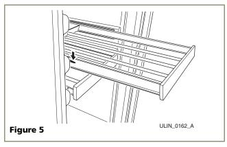
Press the left rack release lever (Figure 5) down, and at the same time, lift the corresponding right rack release lever up, and pull the rack out until it is free of the tracks and the cabinet.
