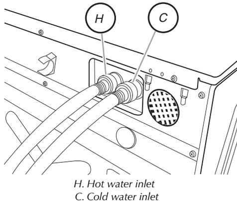
5. Using pliers, check the tightness of the hose couplings already attached to the washer.
