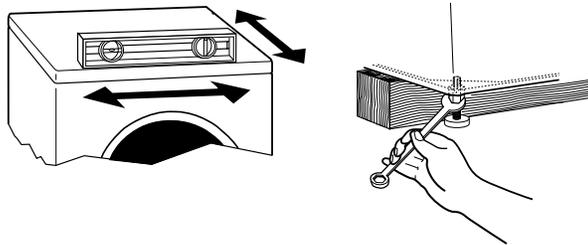
If the washer is against a wall, move the washer out slightly before tipping back. If the washer is not level, first prop the front with a wood block and adjust the feet as necessary; then prop the back and adjust feet as necessary. Repeat this step until washer is level.
