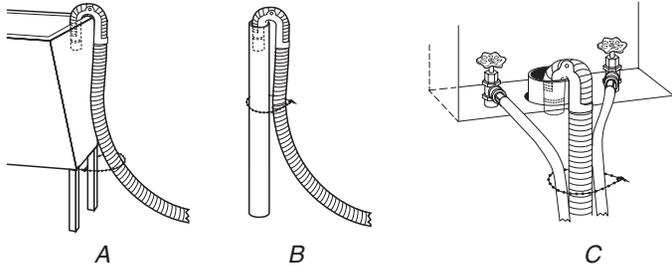
If the washer faucets and the drain standpipe are recessed (see illustration C), put the hooked end of the drain hose in the standpipe. Tightly wrap the beaded strap around the water inlet hoses and the drain hose.
