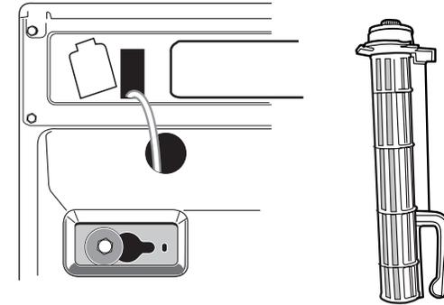
1. Using a 13 mm wrench, loosen each of the bolts.
