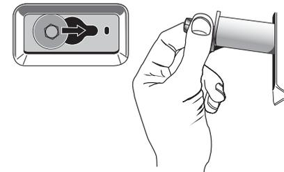
3. Once all 4 bolts are removed, discard bolt and spacers. Then pull the power cord through the opening of the rear panel and close the hole with the attached cap.
