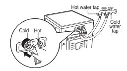
valve on the wall and that cold is connected to cold. The hot water hose has a red stripe, the cold has a blue stripe.
