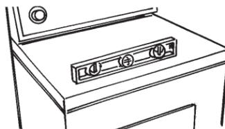
2. Check levelness of dryer by placing a level on top of dryer, first side to side, then front to back. If dryer is not level, adjust dryer legs up or down.
