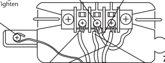
8. Place the hooked ends of the other power supply cable wires under the outer terminal block screws (hook facing right). Squeeze hooked ends together. Tighten screws.
