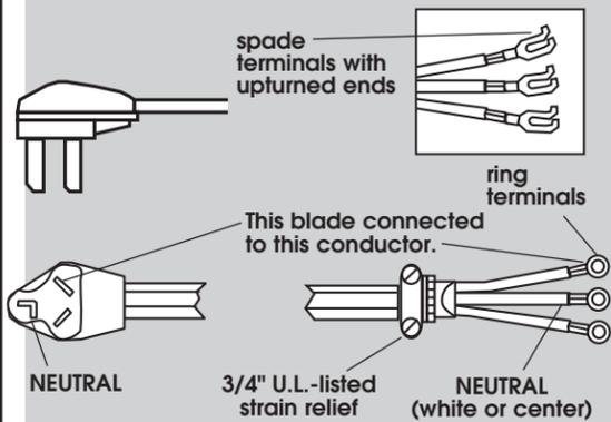
Three-wire power supply cord at least four feet long must have three, No.-10 copper wires and match a three-wire receptacle of NEMA Type 10-30R.
