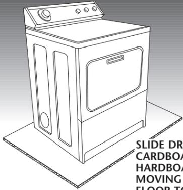
SLIDE DRYER ONTO CARDBOARD OR HARDBOARD BEFORE MOVING ACROSS FLOOR TO PREVENT FLOOR DAMAGE.
