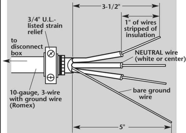
Direct wire cable must have four feet of extra length so dryer can be moved if needed. Strip 5 inches of outer covering from end of cable. Leave bare ground wire at 5 inches. Cut 1-1/2 inches from 3 remaining wires. Strip insulation back 1 inch.
