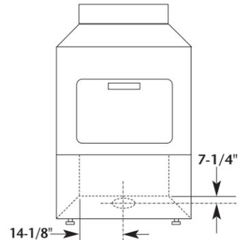
\*Most models will require at least 5" clearance behind the dryer for the dryer vent.
