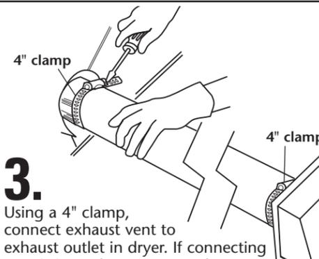
3. Using a 4" clamp, connect exhaust vent to exhaust outlet in dryer. If connecting to existing exhaust vent, make sure the vent is clean. The dryer exhaust vent **must** fit over the dryer exhaust outlet and inside the exhaust hood. Make sure exhaust vent is secured to exhaust hood with a 4" clamp.
