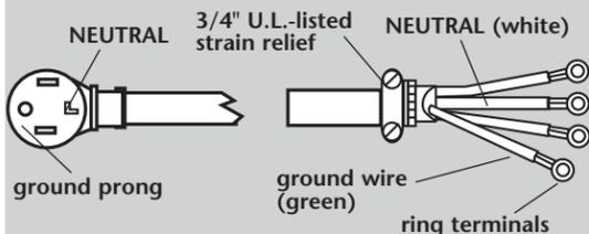
Four-wire power supply cord at least four feet long must have four, No.-10 copper wires and match a four-wire receptacle of NEMA Type 14-30R. The fourth wire (ground conductor) must be identified with a green cover and the neutral conductor by a white cover.
