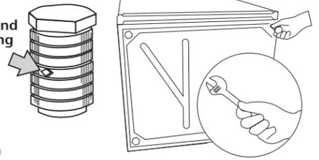
3. Start to screw legs into holes by hand. Use an adjustable wrench or 1" hex-head socket wrench to finish turning legs until you reach the ridge with the diamond marking.
