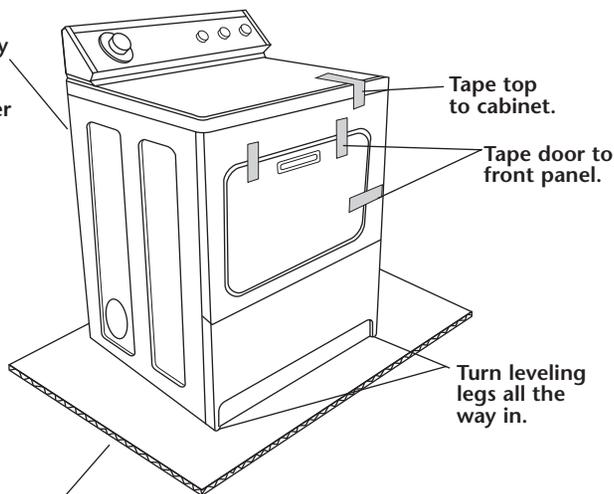
Slide dryer onto cardboard or hardboard before moving it across the floor to prevent damaging floor covering.
