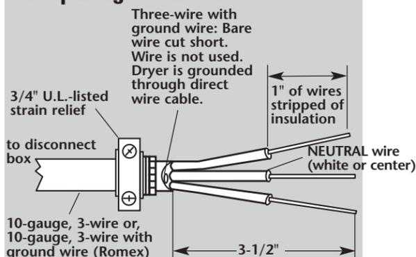
Direct wire cable must have four feet of extra length so dryer can be moved if needed. Strip 3-1/2 inches of outer covering from end of cable. Strip insulation back 1 inch. If using 3-wire cable with ground wire, cut bare wire even with outer covering.
