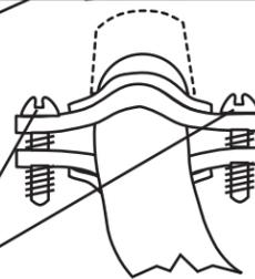
7. Place the hooked end of the neutral wire (white or center) of power supply cable under the center screw of terminal block (hook facing right). Squeeze hook end together. Tighten screw.
