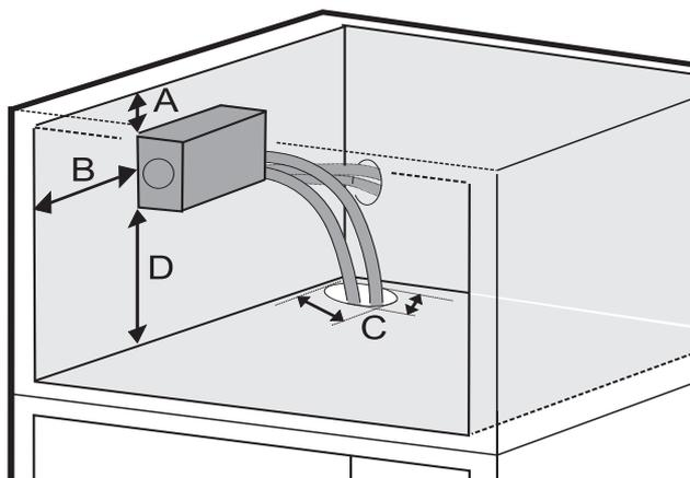
Maintain the dimensions shown in Fig. so that the filter can be replaced and the cover can be removed.
