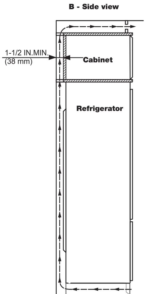
The refrigerator is designed to allow proper air flow when the appliance is installed up against the wall. A minimum space of 1 1/2" (38mm) is required when a cabinet is built above.
