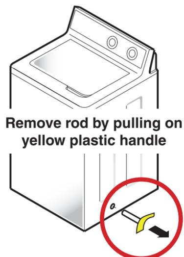
**Avoid a Repair!** Remove metal rod. Leaving rod in place WILL result in severe damage to the washer
