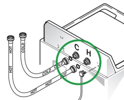
**Avoid a Repair!** Do not cross thread the water hoses and do not forget to install the washers. Flooding may occur
