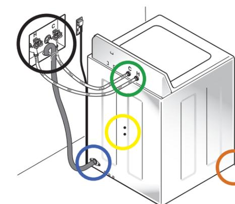
**Avoid a Repair!** Check for leaks after you turn on the water
