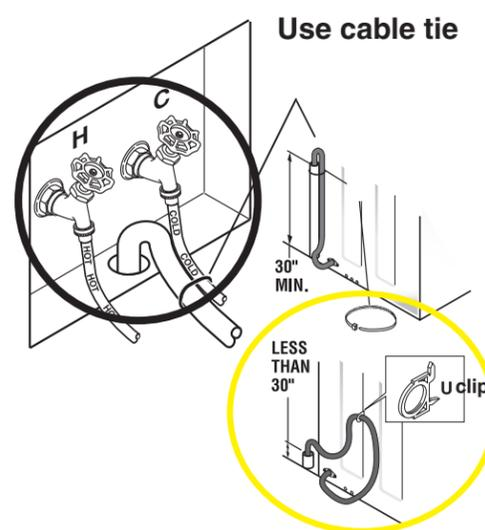
**Avoid a Repair!** Meet 30" drain hose height requirement. Less than 30" without U clip WILL NOT allow proper washer operation
