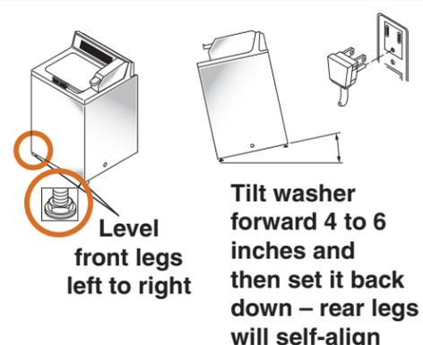
**Avoid a Repair!** Ensure washer is properly leveled, otherwise damage WILL occur
