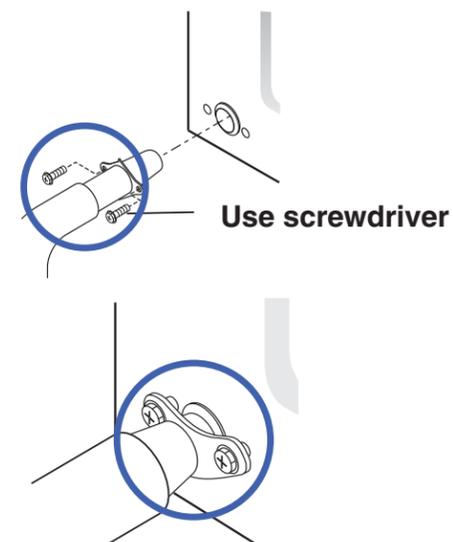
**Avoid a Repair!** Use clamps and screws for drain hose installation; without them leaks and flooding may occur
