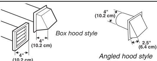
**NOTE:** Side and bottom exhaust installations have a 90° turn inside the dryer. To determine maximum exhaust length, add one 90° turn to the chart.
