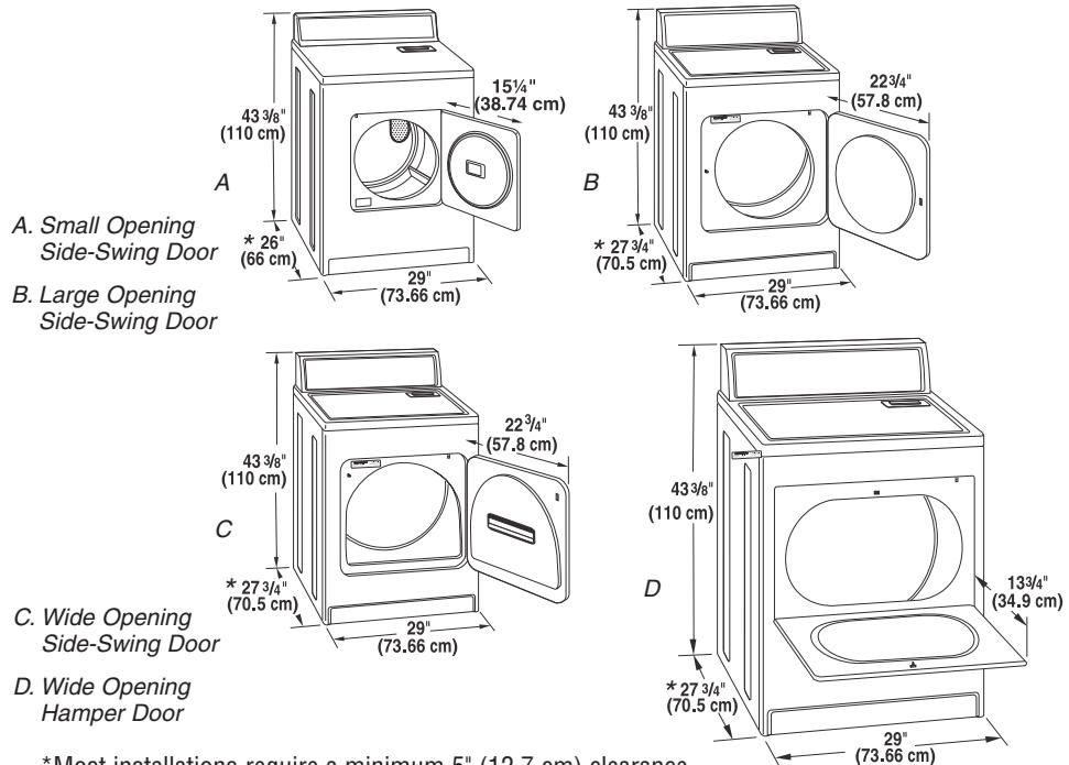
\*Most installations require a minimum 5" (12.7 cm) clearance behind the dryer for the exhaust vent with elbow.
