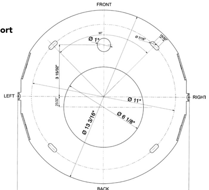
The hole in the ceiling for the ductwork should not be centered over the exact center of the cooking surface as the duct work that runs up inside the chimney and through the ceiling is not in the exact center of the chimney.
