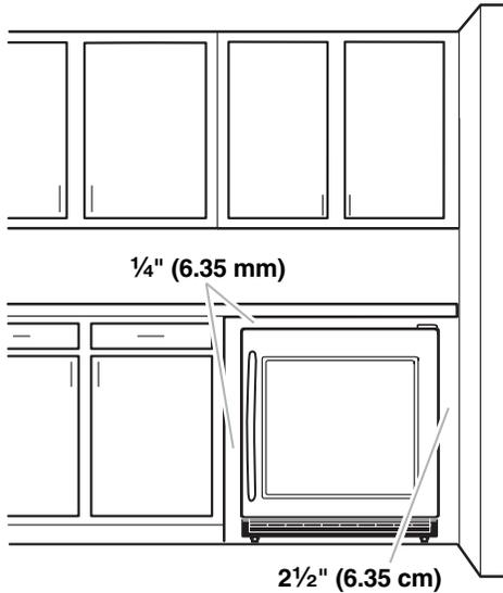
To ensure proper ventilation for your wine cellar, allow for a 1/4" (6.35 mm) space on each side and at the top. When installing your wine cellar next to a fixed wall, leave 2 1/2" (6.35 cm) minimum clearance on each side to allow for the door to swing open.
