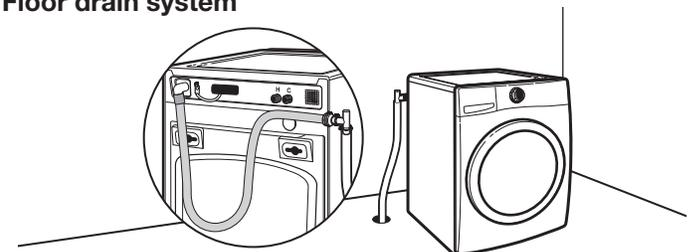
Floor drain system requires a Siphon Break Kit (Part Number 285834), 2 Connector Kits (Part Number 285835), and an Extension Drain Hose (Part Number 285863) that may be purchased separately. See "Alternate Parts". Minimum siphon break height: 28" (710 mm) from bottom of washer. (Additional hoses may be needed.)
