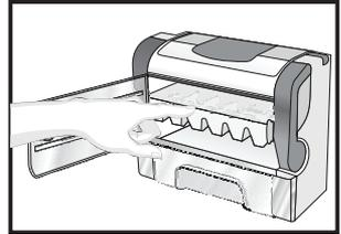
**important:** Use tepid water to remove residual ice which will form with regular use of the Smart Fill Ice Factory. This residue could form on the lid you use to fill the water cylinder, the cylinder valve, and the ice-box, thus affecting the working of different parts of the system.
