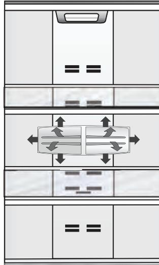
**note:** The Smart Station comes with an air conductor which brings cold air from the freezer to the Smart Station guaranteeing the perfect temperature for your favourite foods.
