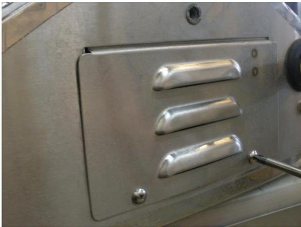
Remove screws from right end Access Cover
