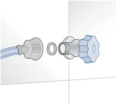
The models provided with Ice Maker require a connection to the domestic water supply system. This can be executed through the provided water hose with 3/4" threading.
