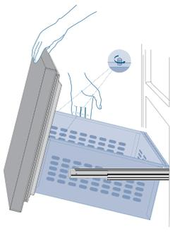
The upper TriMode can be removed using the same method used for the Fresco drawer
