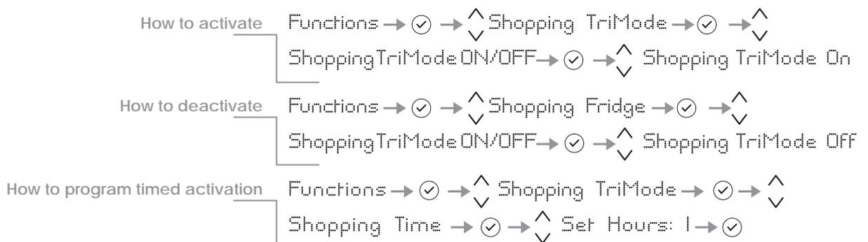
It is possible to program the function with a delay of 1 to 12 hours.
