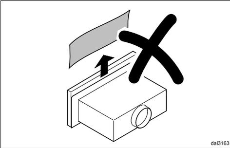
To avoid scratching the deflector plate, do not remove the protective film between the deflector plate and the casing until the rangehood has been placed in the housing unit.
