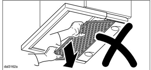
When removing the grease filter do not tilt it downwards at an angle. This can damage the retaining pins.
