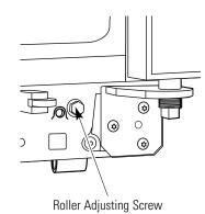
• Use a 3/8" hex socket or wrench to turn the adjustment screws. Turn the screws clockwise to raise the refrigerator, turn counterclockwise to
