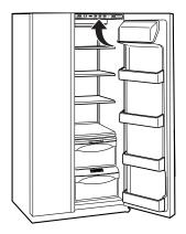
The temperature controls are preset in the factory at 37°F for the fresh food compartment and 0°F for the freezer compartment. Allow 24 hours for the temperature to stabilize to the preset recommended settings.
