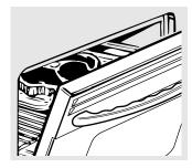
If your oven is connected to 208 volts, rare steaks may be broiled by preheating the broiler and positioning the oven rack one position higher.
