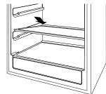
Place in slots when replacing the shelf
