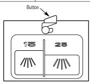
To open the wash cover, press the button and the cover will flip back.
