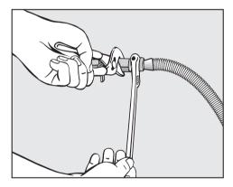
Using two adjustable wrenches tighten all connections.
