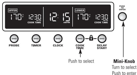
**Timed cooking allows you to set the oven to turn on immediately, cook for a selected length of time and turn off automatically.**
