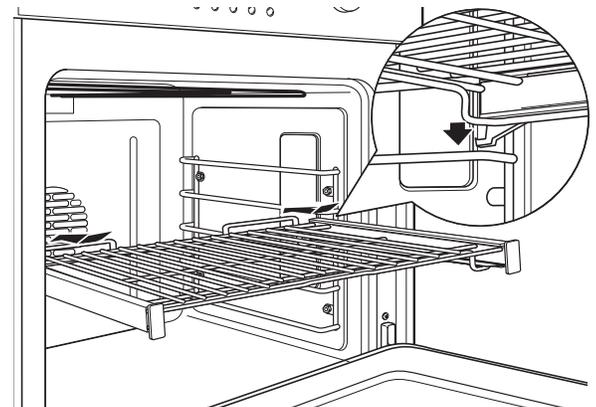
2. Slide the rack all the way in until the rear rack locks are secure on the rear rack supports and press the front rack locks onto the front rack supports.
