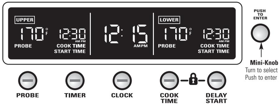
Push the **PROBE**, **TIMER**, **CLOCK**, **COOK TIME** or **DELAY START** buttons and set them by turning and pushing the Mini-Knob. See each respective section for details.
