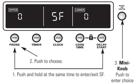
5 Push and hold the Mini-Knob for 5 seconds to exit SF (Special Features) and return to the time of day clock.
