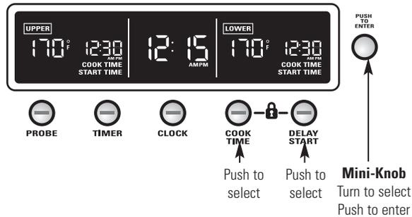
**Timed cooking with DELAY START allows you to set the oven to turn on at the time of day you set, cook for a selected length of time and turn off automatically.** DELAY START cannot be used with the Sabbath feature.
