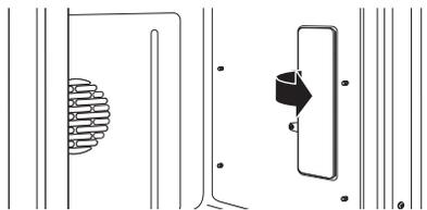
**NOTE:** The two locking clips may fall from the glass light cover. Upon replacement, they will need to be placed in the correct position on the light cover and pressed back into the light compartment until seated.
