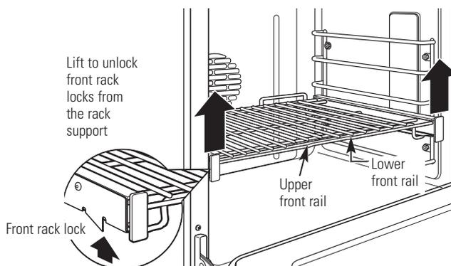
3. Firmly holding onto both the upper and lower front rack rails, pull the rack forward and remove it from the oven.
