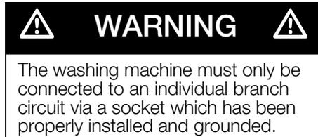
The household electrical voltage must correspond to the voltage specification on the washing machine (rating plate, see page 31).
