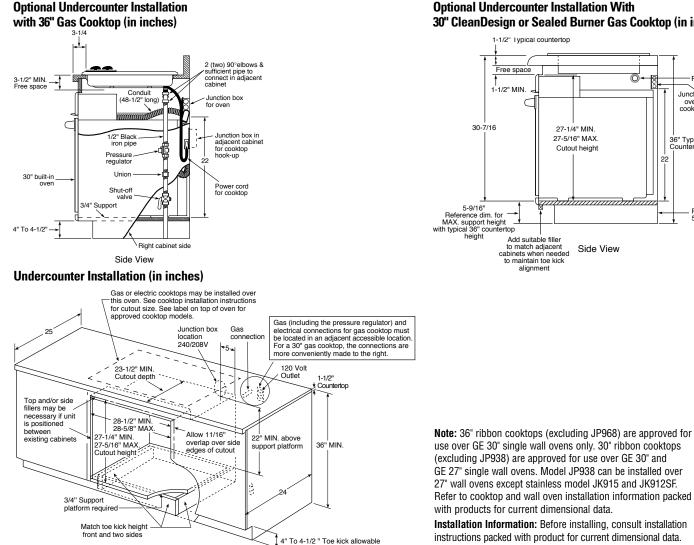
**Optional Undercounter Installation With** 30" CleanDesign or Sealed Burner Gas Cooktop (in inches)
