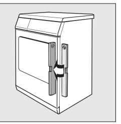
The dryer must be level to ensure safe and proper operation.
