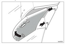
Hook the decor cover on to the latches on the rear panel of the chimney. Push the cover up at the front so that it clicks in place.
