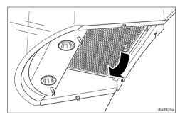
■ To remove the grease filter, pull on the release knob. Hold the grease filter when doing this so that it does not fall on to the cooktop.
