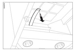
Before inserting an active charcoal filter for the first time remove the connector for use in air extraction mode. Loosen the screw in the connector and remove.
