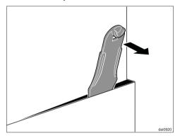
■ After removing the screws from the chimney, slide the lever between the chimney and the chimney extension and gently apply pressure to ease the chimney from its hooks.
