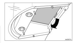
■ To remove the active charcoal filter pull down on the tab at the back of the filter.
