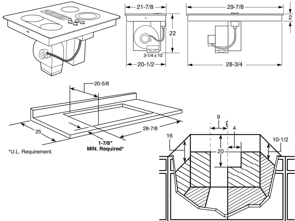
\*Note: A 6" minimum spacing to adjacent side wall is required. Dimension and installation information are shown in inches.
