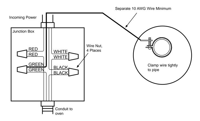
**Three Wire Connection with External Ground**
