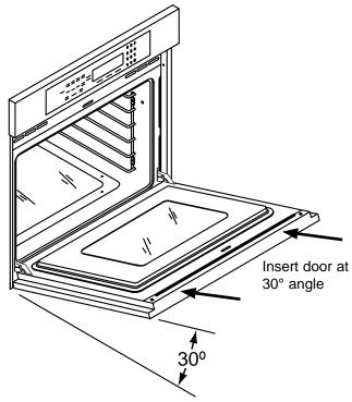
3. Lower the door to the fully opened position. Rotate <u>both</u> hinge catches toward the oven. Open and close the door slowly and completely to ensure that it is properly installed.
