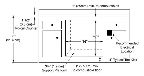
Single Wall Oven - Installed Under Counter
