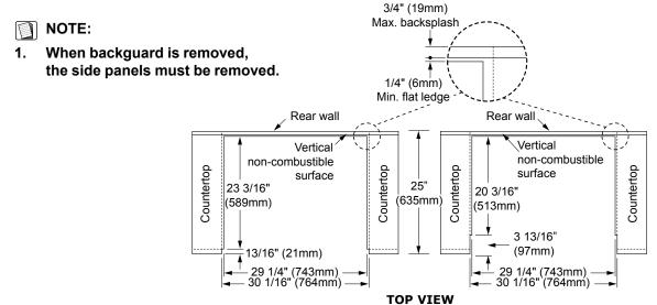
(Slide-In, Self-Rimming Installation with Side Panels and Backguard Removed)
