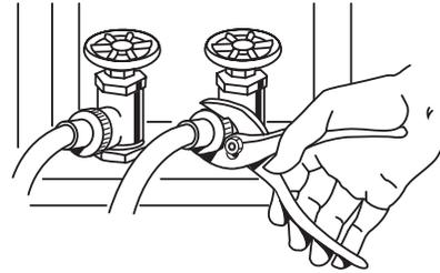
**NOTE:** Do not overtighten. Damage to the coupling can result.
