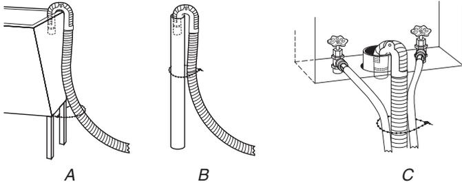
If the washer faucets and the drain standpipe are recessed (see illustration C), put the hooked end of the drain hose in the standpipe. Tightly wrap the beaded strap around the water inlet hoses and the drain hose.
